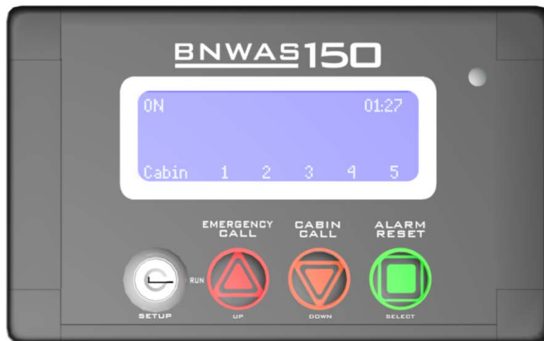
Figure 1 - DC-150 Control Display Panel
